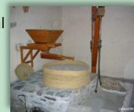
**1-Mill of Sevillano** - Mill for the study of water, shows how the grain is ground using the mechanical force of water.
